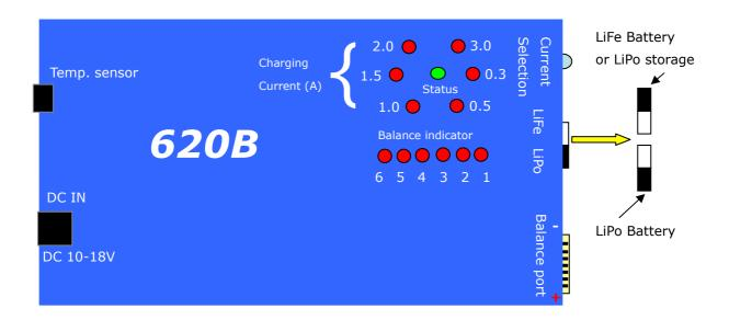
There is a **Current Selection button** on the right of the CY-620B, press the button to choose the charging current, 6 types of current is be used for the different capacity, we suggest the charging current is no more than 1C, if the battery capacity is 1000mAh, the charging current is lower than 1000mA.
